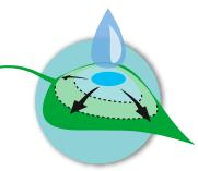
EXPANSION HURRICANE reduces the surface tension of droplets (reduced from 60/70 dyn/cm to 32/35 dyn/cm). As a result, the surface coverage of the sheet is better.
